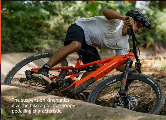
The E-160 layout is familiar but the mainframe is all new for increased stiffness, and easier, bigger battery management.
